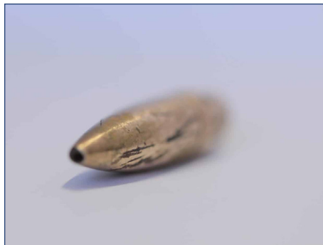
Figure 5. An open-tip 7.62mm bullet found by Forensic Architecture’s researchers in Gaza during the 2018 Great March of Return, highly suspected to be from Sierra Bullets. 64
